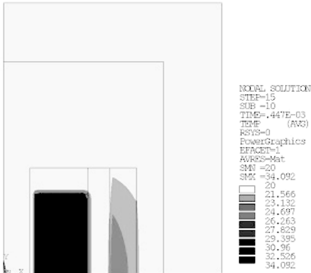
Fig. 4. Distribution of temperature at the end of the first load t = 0.447 ms
