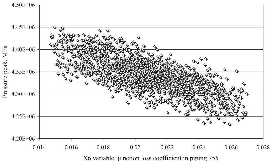
Fig. 4. Scatter plot of X6 against the model output (pressure peak)
