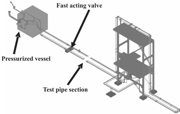
Fig. 1. Perspective view of pilot plant pipework [4]
