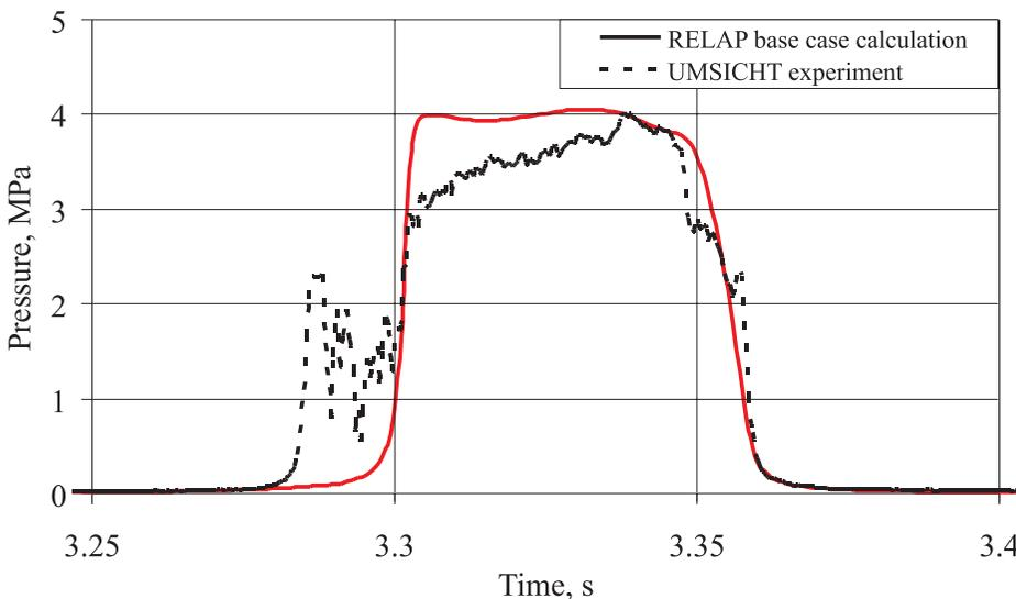
Fig. 3. Comparison of the RELAP5 basic case calculation with UMSICHT experimental data
