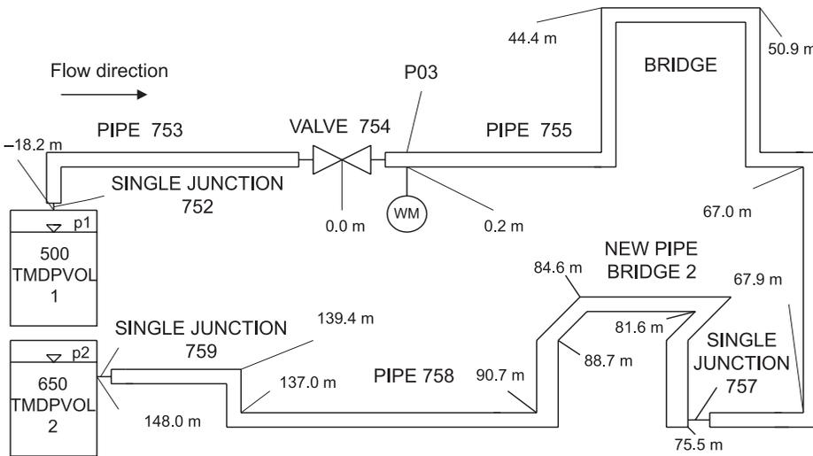
Fig. 2. Pilot plant pipework (UMSICHT) RELAP5 / Mod3.3 code model nodalization scheme
