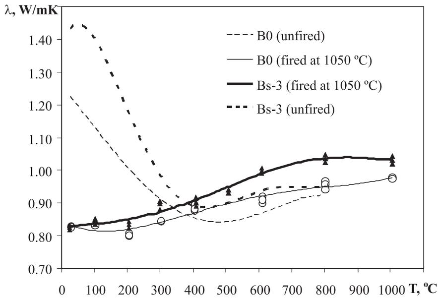
Fig. 2. Comparison of thermal conductivity of unfired and sintered refractory castable
