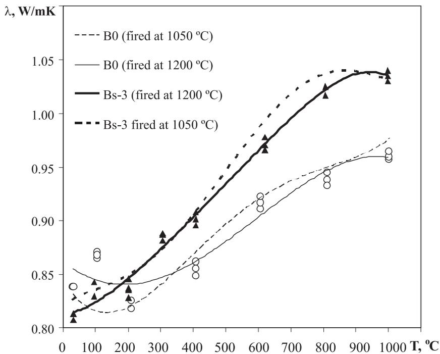
Fig. 3. Thermal conductivity of sintered at different temperatures refractory castable as a function of temperature.
