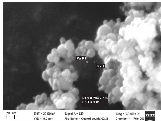
Fig. 1. SEM image of RW-Fuller microsilica
