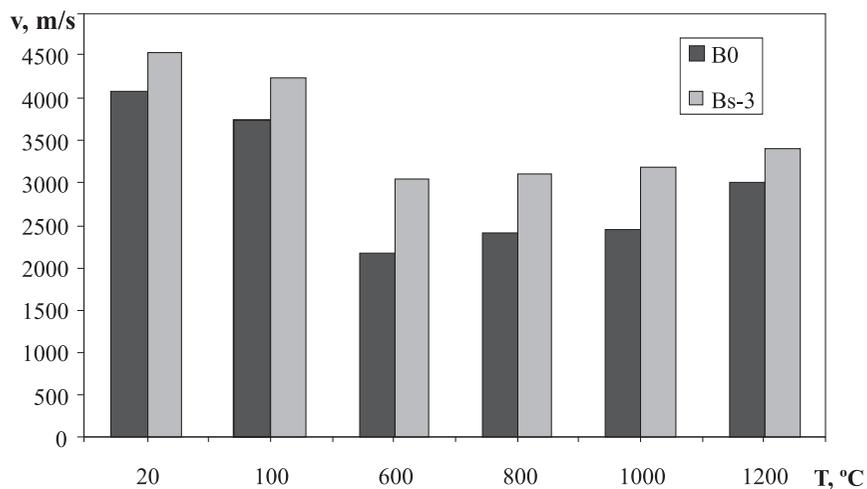
Fig. 4. Ultrasonic wave (UW) velocity in samples of castable
