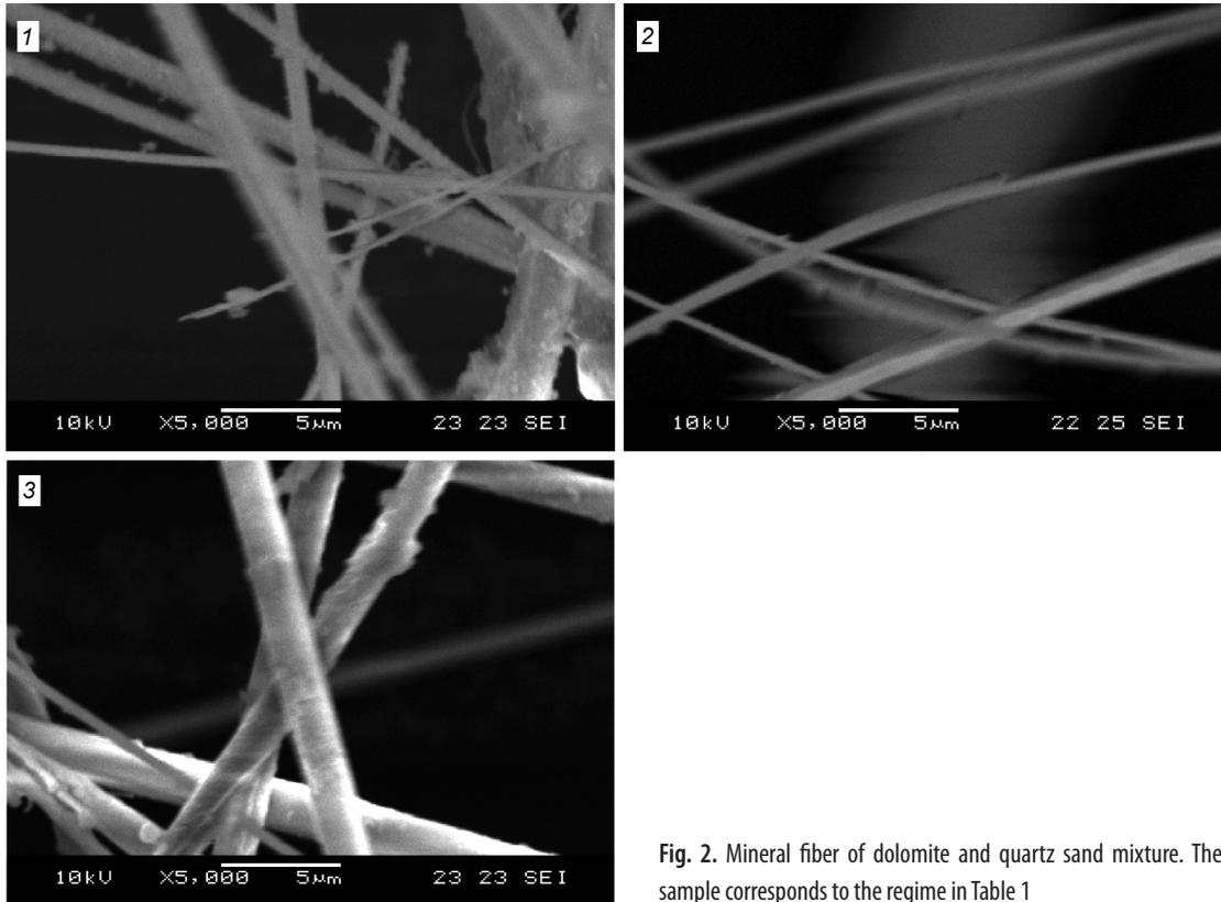
Fig. 2. Mineral fiber of dolomite and quartz sand mixture. The number of sample corresponds to the regime in Table 1
