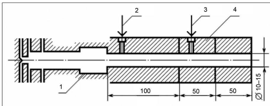
Fig. 1. Schematic presentation of uniflow plasma-chemical reactor: 1 – plasma torch, 2 – injection place of raw material, 3 – additional gas feeding, 4 – transformable reactor sections
