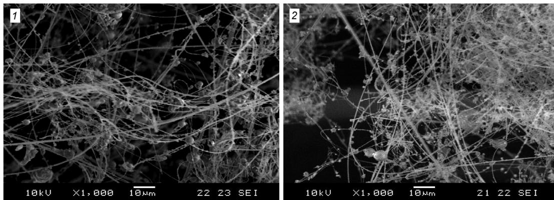
Fig. 3. Mineral fibers obtained with different outlet exhaust diameters: 1 – 0.015 m, 2 – 0.010 m
