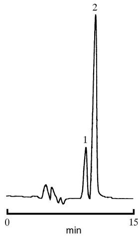
Fig. 5. Chromatogram of 1:10 diluted beverage "Natūralūs gėrimai" sample. Peaks: 1 – benzoate, 2 – sorbate. Other conditions as in Fig. 4
