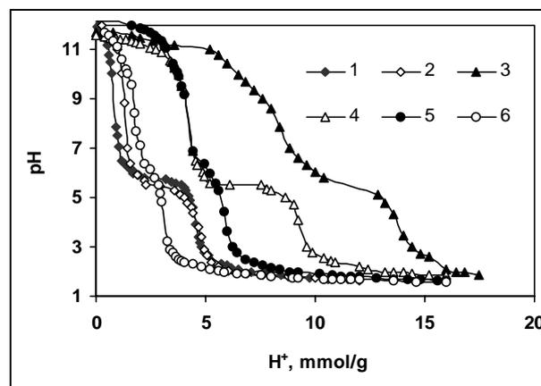
Fig. 1. pH-metric titration of chitosan suspensions. The number of curves corresponds to the number of chitosans from Table 1
