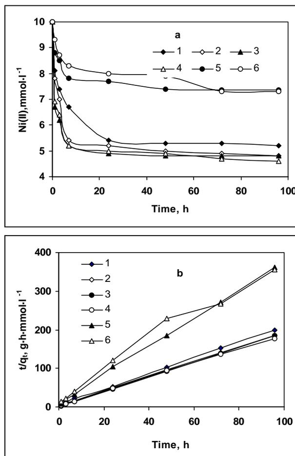
Fig. 3. The uptake of Ni(II) by chitosans. Initial concentrations  $10\text{ mmol} \cdot \text{l}^{-1}$  Ni(II) and  $10\text{ mmol} \cdot \text{l}^{-1}$  citrate, pH 7 (a) and test of pseudo-second order equation for adsorption of Ni(II) (b). Number of curves corresponds to the number of chitosans from Table 1
