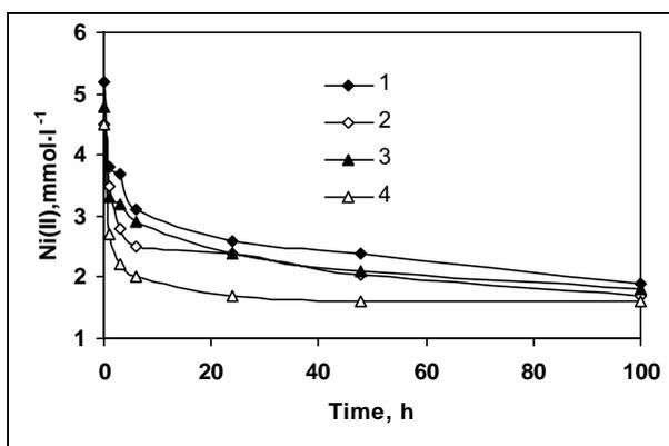
Fig. 5. The second uptake of Ni(II) that remained after treatment under the same conditions as in Fig. 3 with fresh chitosan. The number of curves corresponds to the number of chitosans from Table 1
