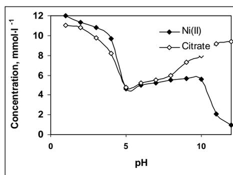
Fig. 2. Influence of pH on the residual concentrations of Ni(II) and citrate after sorption onto chitosan No 4
