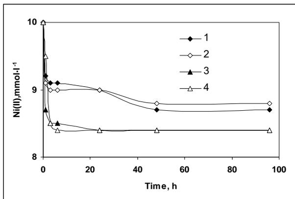
Fig. 4. The uptake of Ni(II) from fresh solution on chitosan once used under conditions of Fig. 3. pH 7. The number of curves corresponds to the number of chitosans from Table 1
