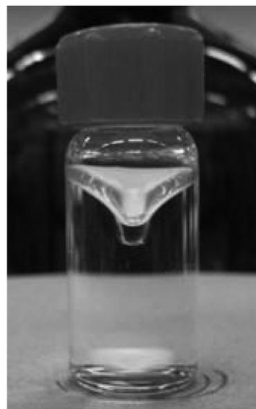
Fig. 1. A Photograph of the DSDME process
