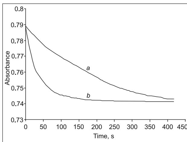
Fig. 6. Time-dependent responses of the optical sensor to a  $1.5 \times 10^{-4} \text{ mol L}^{-1}$  sulfide solution in the absence (A) and presence (B) of  $1.26 \times 10^{-5} \text{ mol L}^{-1}$  of Se(IV)
