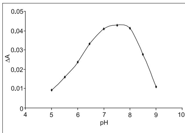
Fig. 7. Effect of pH of test solution of  $1.5 \times 10^{-4} \text{ mol L}^{-1}$  sulfide on the response of membrane optode
