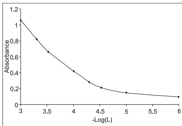
**Fig. 3.** Absorbance of the immobilized agarose membrane at 620 nm as a function of methylene blue concentration during synthesis
