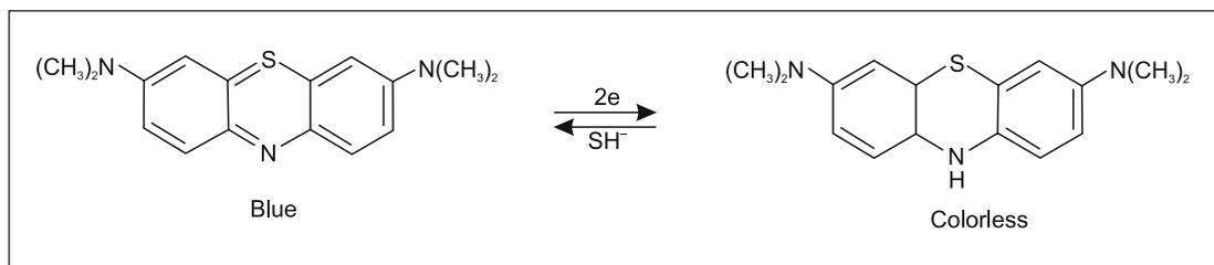
Fig. 5. Reduction reaction of methylene blue by sulfide ion
