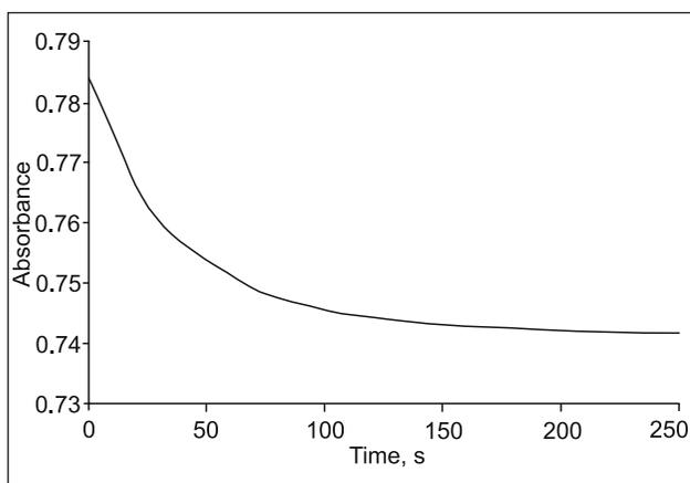
Fig. 8. The absorbance-time plots for the optode membrane in the presence of  $1.5 \times 10^{-4} \text{ mol L}^{-1}$  sulfide
