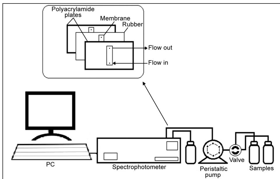
Fig. 1. Set-up of the measuring flow system
