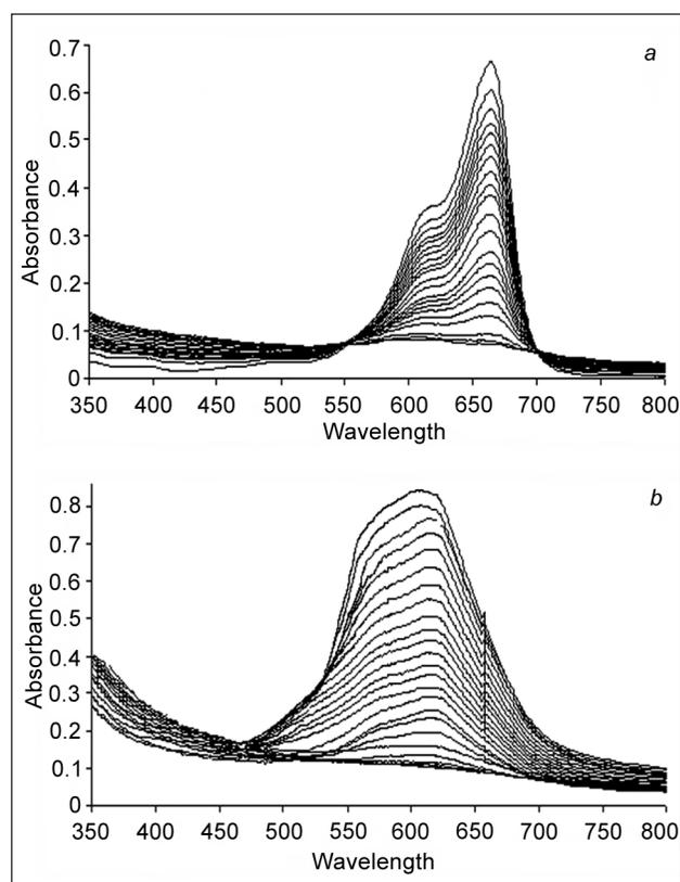
**Fig. 4.** (a) Absorbance spectra of dissolved methylene blue at different sulfide concentration and (b) Absorbance spectra of immobilized methylene blue at different sulfide concentration
