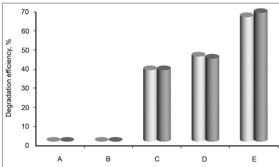
**Fig. 2.** Efficiency of different procedures of imidacloprid photodegradation after 1 hour: without a catalyst / dark regime (A), photolysis (B), unmodified ZnO (C), Ag/ZnO/1 (D), Ag/ZnO/2 (E)
