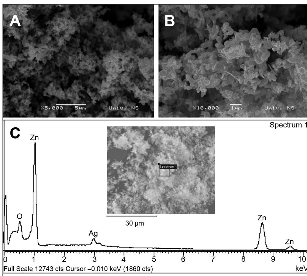
**Fig. 3.** SEM micrographs of the Ag/ZnO/2 sample under different magnifications ( $\times 5,000$  (A),  $\times 10,000$  (B)) and EDS spectra from its representative surface area (C)
