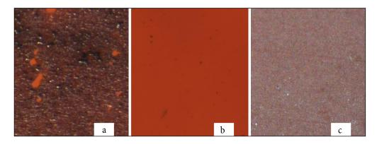
**Fig. 2.** Optical micrograph image of the PA6–Se precursor with top coating (a), cleaned (b) and the PA6–Se–Cd composite (c). Magnification  $\times$ 100
