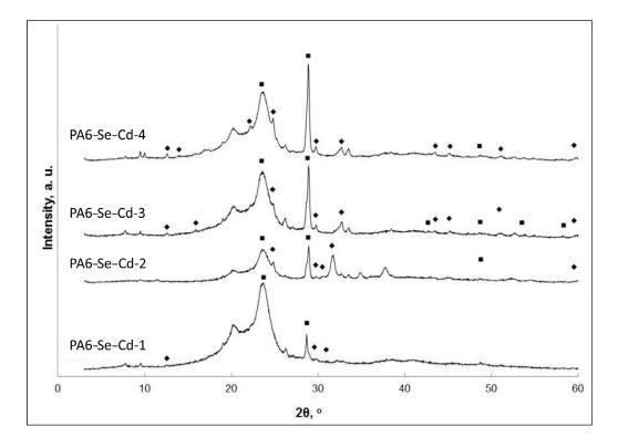
Fig. 3. XRD spectra of the PA6–Se–Cd composites, obtained at a different temperature as indicated in Table 1. ♦ is Se, ■ is CdSe
