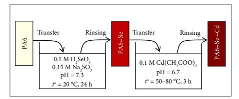
Fig. 1. The principal scheme of PA6–Se–Cd composite synthesis route
