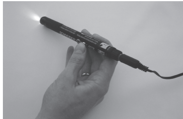
Fig. 1. Fluorescence excitation system based on blue light emitting diode
