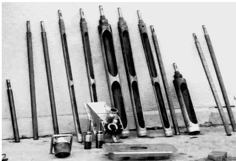
Photo 3. Core probes of the diesel hammer drill (by H. Hajdukiewicz)
