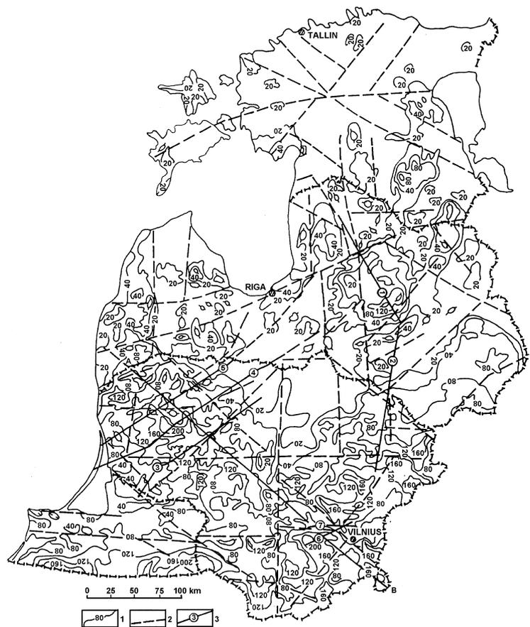
Fig. 3. Thickness of the Quaternary of the Baltic area (after Šliaupa et al., 1987): 1 – Quaternary isopachs, 2 – major faults of the crystalline basement and sedimentary cover (Puura (ed.), 1980), 3 – lines of geological cross-sections
