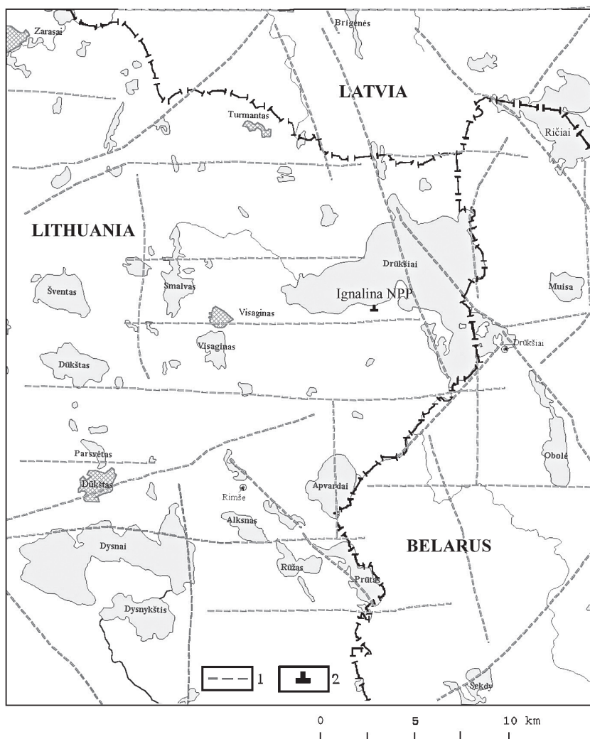
Fig. 5. Neotectonic map of the Ignalina NPP area (A. Šliaupa, 1995): 1 – neotectonic active linear zones; 2 – Ignalina NPP
