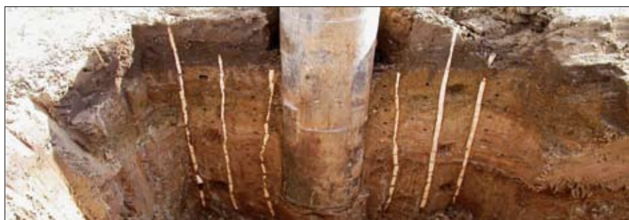
Fig. 6. The excavation intended for performing the measurement and soil sampling 6 pav. Kasinys matavimams ir bandiniams
