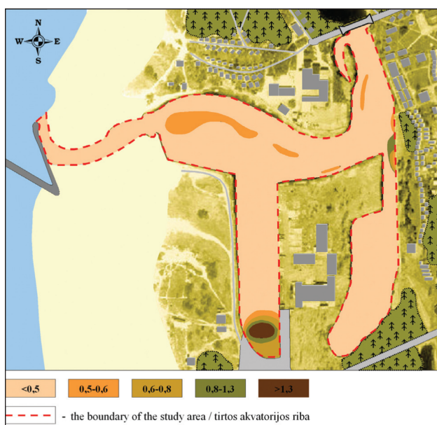
Fig. 17. Cadmium (Cd) concentration (mg/kg) in the bottom sediments (0–5 cm) of Šventoji Port
