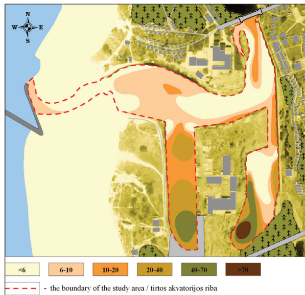
Fig. 15. Lead (Pb) concentration (mg/kg) in the bottom sediments (0–5 cm) of Šventoji Port
