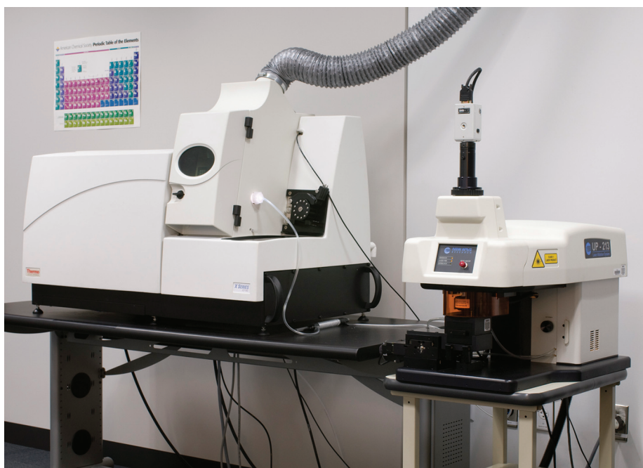
Fig. 4. The need for accurate chemical composition data for minor and trace elements in gem materials has resulted in major gemological laboratories acquiring equipment capable of analyzing materials using the laser ablation – inductively coupled plasma – mass spectrometry (LA-ICP-MS) technique. Shown here are a Thermo X Series II ICP mass spectrometer on the left, and a New Wave UP-213 laser ablation system on the right. Photo by Kevin Schumacher, copyright GIA 4 pav. LAICPMS sistema
