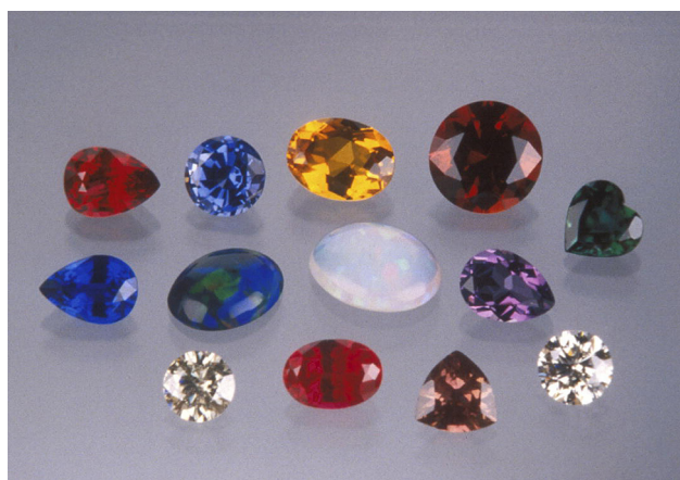
Fig. 2. A variety of synthetic gem materials can be found today in the jewelry marketplace. From left to right starting at the top row, these include synthetic red spinel, synthetic blue sapphire, synthetic citrine, synthetic red beryl, synthetic emerald, synthetic blue spinel, two synthetic opals, synthetic amethyst, synthetic moissanite, synthetic ruby, synthetic alexandrite, and a synthetic diamond. The items weight from 0.43 to 1.81 carats. Photo by Maha Tannous, copyright GIA
