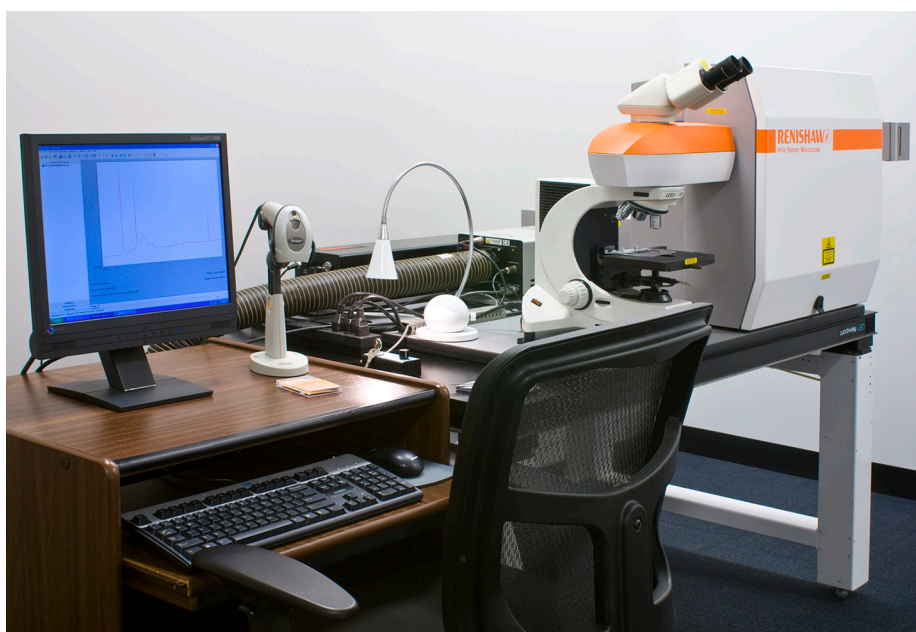
Fig. 3. This Renishaw 1000 InVia Raman microscope allows the collection of both Raman spectra as well as photoluminescence spectra of a gem material. The equipment is set up to use several lasers with different excitation wavelengths (488.0, 514, 633 and 830 nm). Photo by Kevin Schumacher, copyright GIA 3 pav. Raman spektroskopijos sistema
