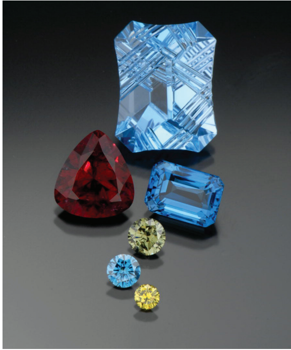
Fig. 1. These gemstones were all treated by radiation exposure in the laboratory to improve their color. The group includes two examples of irradiated blue topaz (33.75 and 9.12 ct.), an irradiated red tourmaline (6.97 ct.), and three irradiated colored diamonds (0.50–0.80 ct.). Photo by Robert Weldon, copyright GIA 1 pav. Švitinti brangieji ir juvelyriniai mineralai
