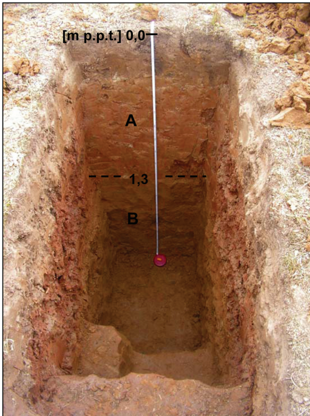
Fig. 2. Exploration pit where polluted soil was sampled. A – upper till horizon, thickness about 1.3 m, brown-red clayey till with few pebbles, B – lower till horizon, analysed brown sandy till
