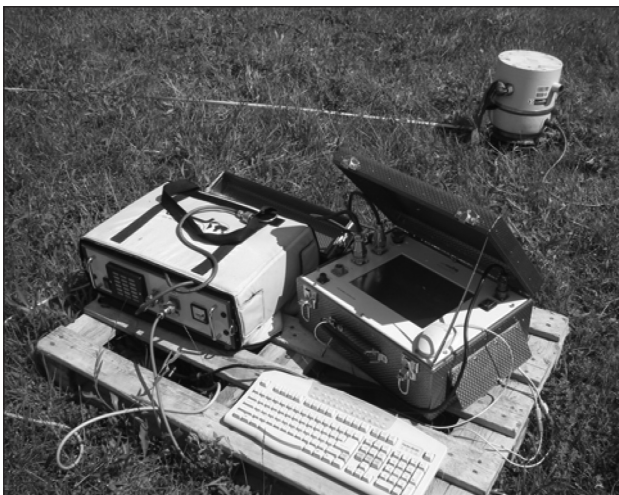
Fig. 4. Part of a seismic system. Control units (foreground), vibrator (background). Geophones not visible
