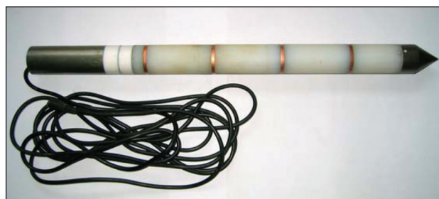
Fig. 5. Prototype geoelectrical probe for electrical soil resistance
