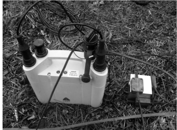
Fig. 2. Seismic station and XYZ three-component geophone set
