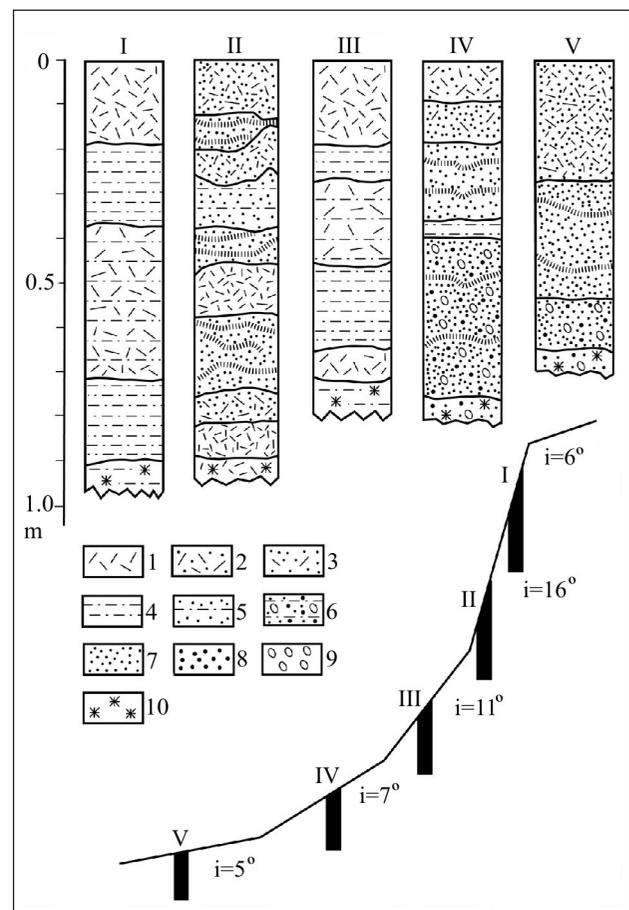
Fig. 3. Position of the boreholes on the slope: 1 – peat, 2 – sandy peat, 3 – sand with organic, 4 – silt, 5 – silty sand, 6 – pebbles, gravel, sand and silt, 7 – sand, 8 – gravel, 9 – pebbles, 10 – permafrost
