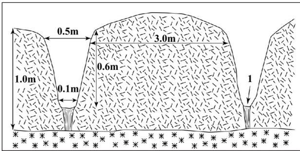
Fig. 6. Cross-section of permafrost surface: 1 – ice wedge
