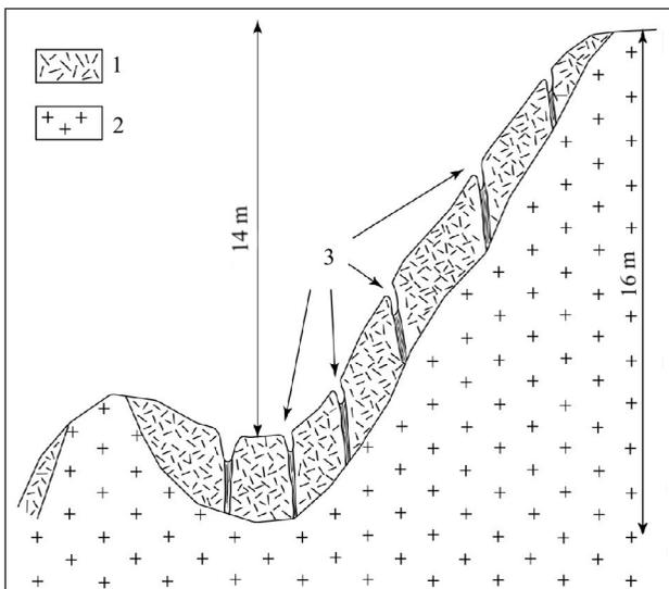
Fig. 7. Cross-section of permafrost surface on the slope: 1 – peat, 2 – magmatic rocks, 3 – ice wedge
