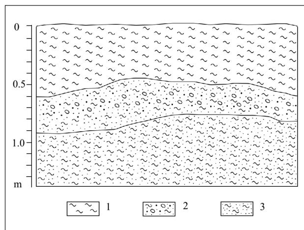
Fig. 10. Typical scheme of a deflation outcrop: 1 – silt, 2 – pebbles, gravel, sand and silt, 3 – silty sand
