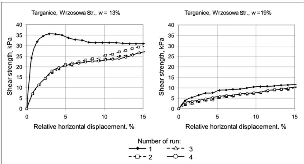
Fig. 4. Examples of relationships between shear strength and relative deformation of soil (normal stress 25 kPa)
