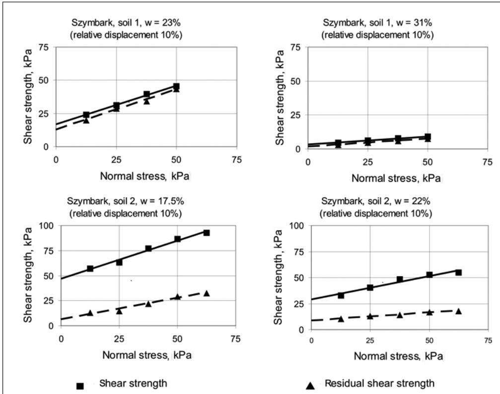
Fig. 3. Shear strength of soils from Beskid Niski
