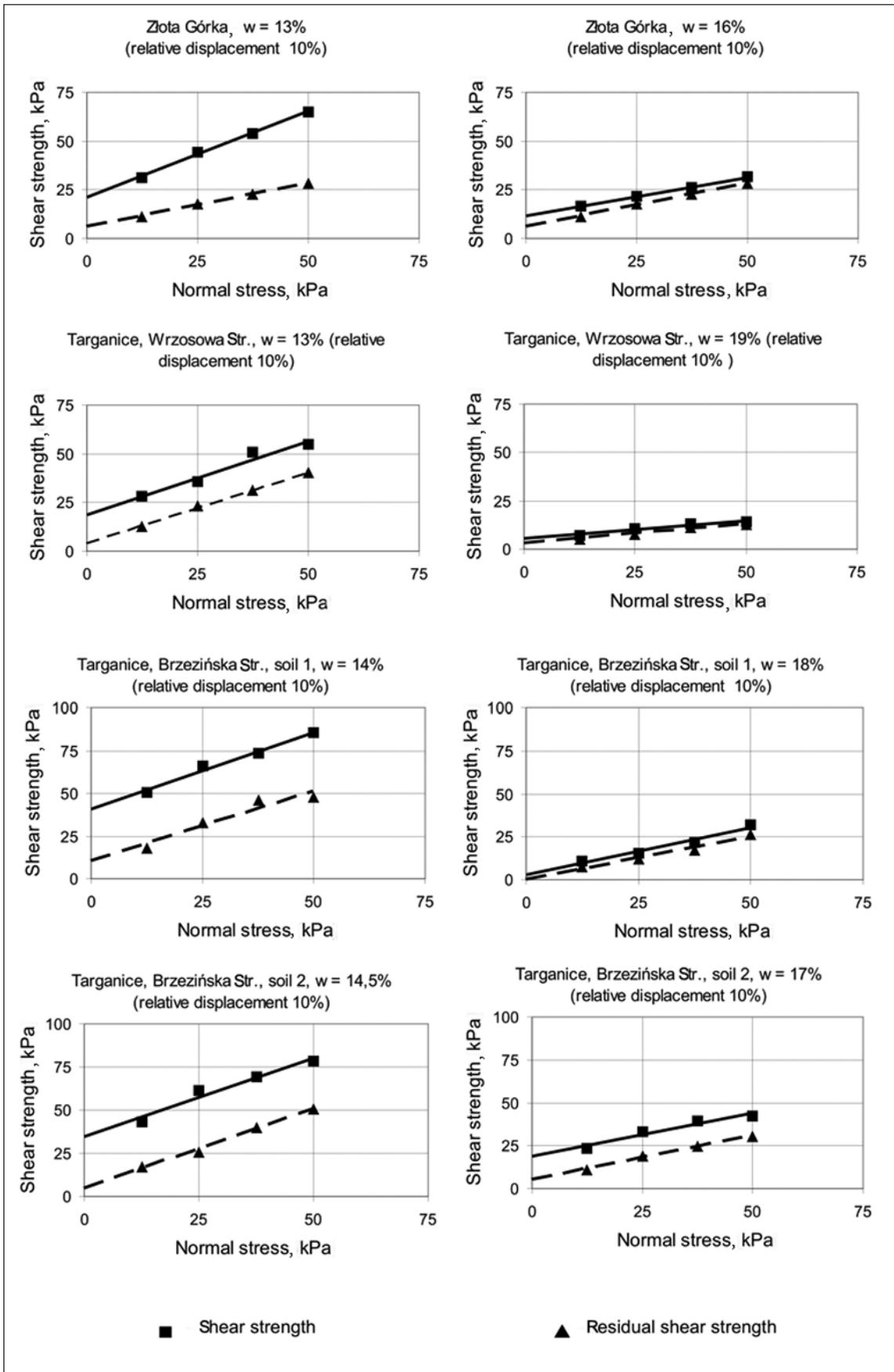
Fig. 2. Shear strength of soils from Beskid Mały
