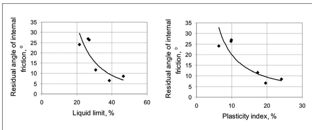
Fig. 5. Relationships of obtained residual values of the angle of internal friction versus liquid limit and plasticity index of test soils
